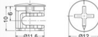
MF-105 Casing Minifix Material : Zinc Alloy
